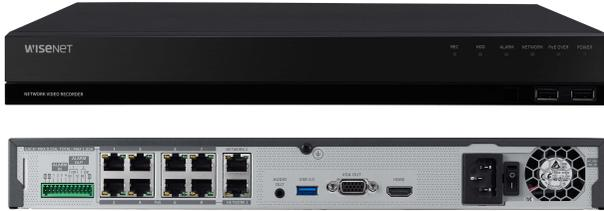
The WRN-810S is a Wisenet WAVE optimized 1U rackmounted Network Video Recorder capable of recording up to 80Mbps, managing up to 12TB of storage. The Linux Ubuntu OS is utilized for stability and quick setup.
